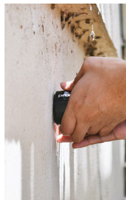
AMH team performs Ultrasonic Pulse Velocity (UPV) test during March 2 to 5, 2020 ocular inspection. Photograph by Engr. Mary Grace Casuncad.
