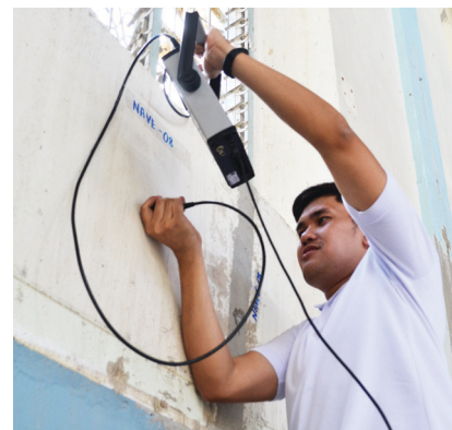
AMH team performs Ultrasonic Pulse Velocity (UPV) test during March 2 to 5, 2020 ocular inspection. Photograph by Engr. Mary Grace Casuncad.
